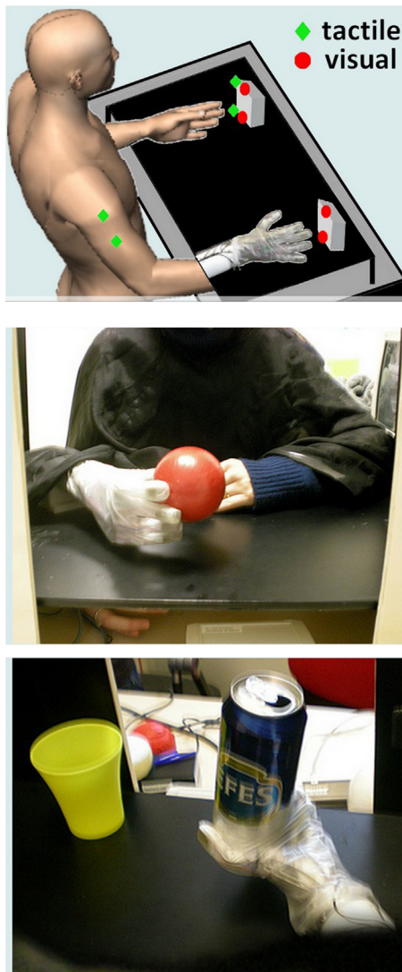
Fig. 1. The upper panel schematically depicts the experimental setup. The participant's left arm is positioned on a table, while his right arm is positioned below an opaque screen in correspondence with the robotic hand. Green diamonds indicate the position of the tactile stimulators: those on the arm (right-side) delivering tactile stimuli during the training ((1) afference from fingers 2–5 and from the palm; (2) afference from the thumb); those on the foam cube (left-side), delivering tactile stimuli during the crossmodal congruency test ((1) position of the index; (2) position of the thumb). Red circles represent visual distracters during the crossmodal congruency test. The middle and lower panels are illustrative pictures from one training session, where the subject is required to perform exercises such as passing a ball between the robotic and the real hand (middle panel) and grasping an empty can with the robotic arm (lower panel). (For interpretation of the references to color in this figure legend, the reader is referred to the web version of this article.)
